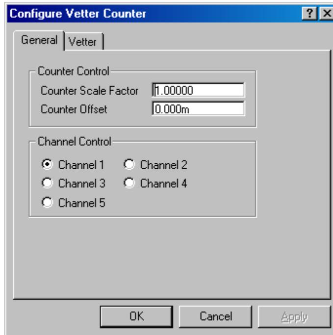
The dialog contains two tabs, General and Vetter. The first allows you to configure basic counter parameters, the second provides configuration of settings particular to the Vetter plus the roll over issue.
